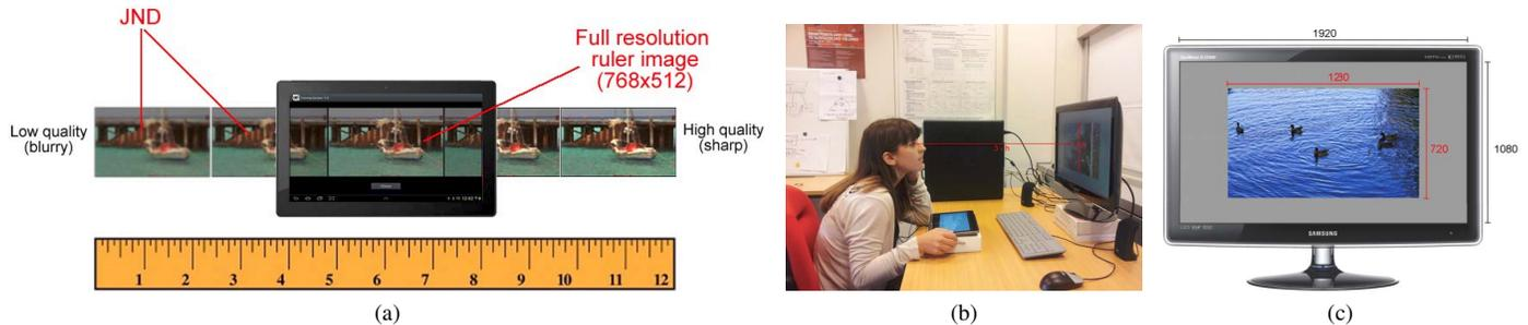
Fig. 2: Parts of the VQR apparatus. (a) Quality ruler implemented on a tablet screen. The images going out to the tablet represent the next or previous reference images. (b) Experimental setup of Video Quality Ruler. (c) Video playing on screen monitor.
